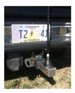
• Connecting a ground strap with a quick connect to the MFJ-2822 is recommended as the hitch does not supply the antenna with a secure ground connection.
